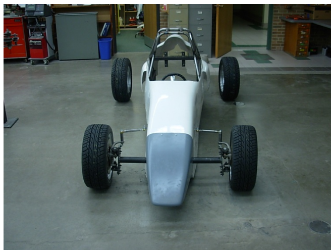
-The Chassis with axle, front wheels, and fiberglass body attached (below)
