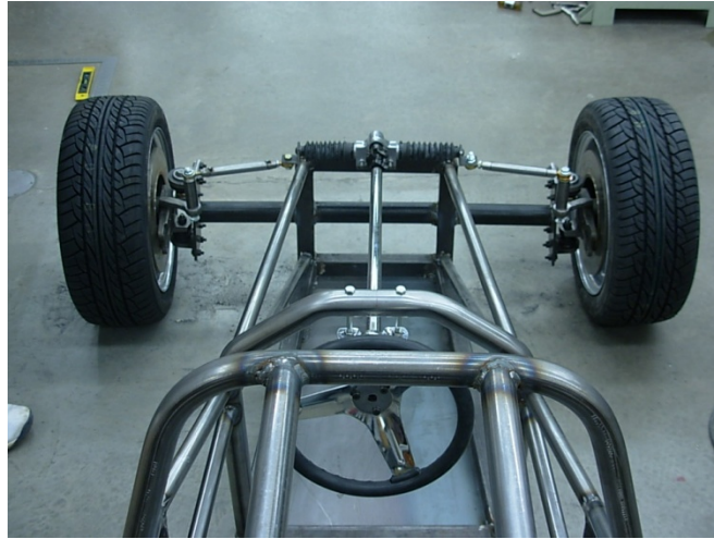
-Full front wheel and axle assembly with steering attachment (back view 1)(above), (back view 2) (below).
